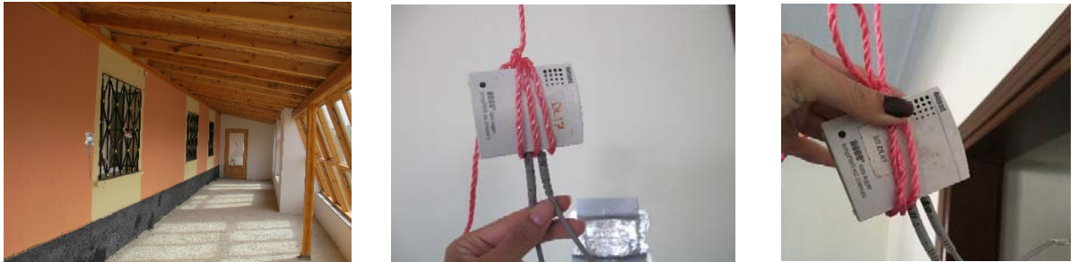
Figure 31. Experiment on thermal performance of the building using data loggers and sensors (2015-2016).
