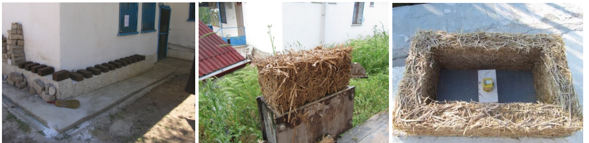
Figure 29. Academic research on local materials and their properties (mud bricks and their additives, 2008, building with lightweight loam and pine-needles, 2013)
