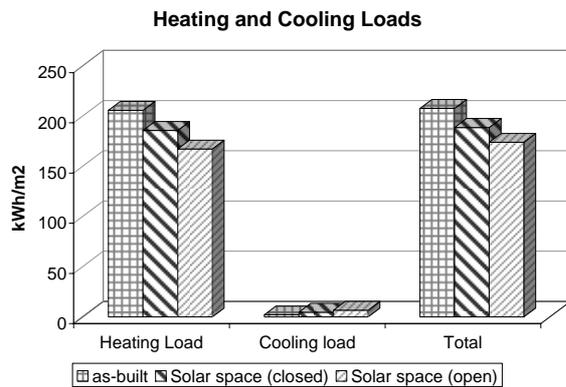
Figure 7: Annual energy loads for the simulated Mud-brick Building; with and without the solar space.
