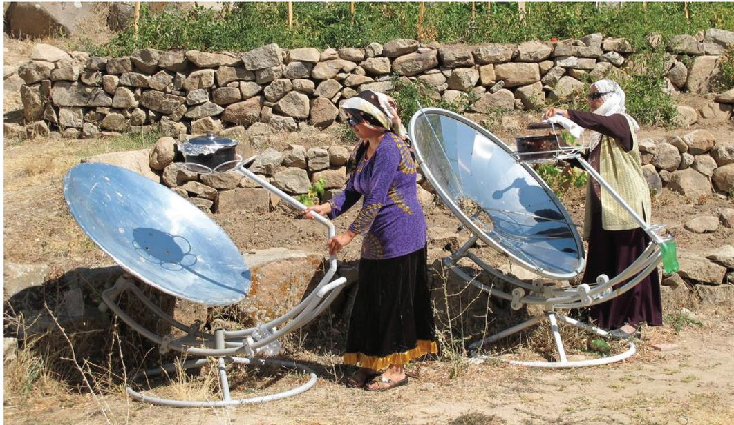
*Figure 13. Parabolic solar cookers used to make jam.*
