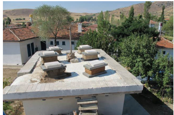
Fig 8: Dataloggers are placed inside boxes made from different materials.
