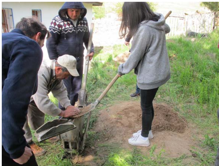
Figure 13. Filling the press with the mud mixture. (18kekc0210)
