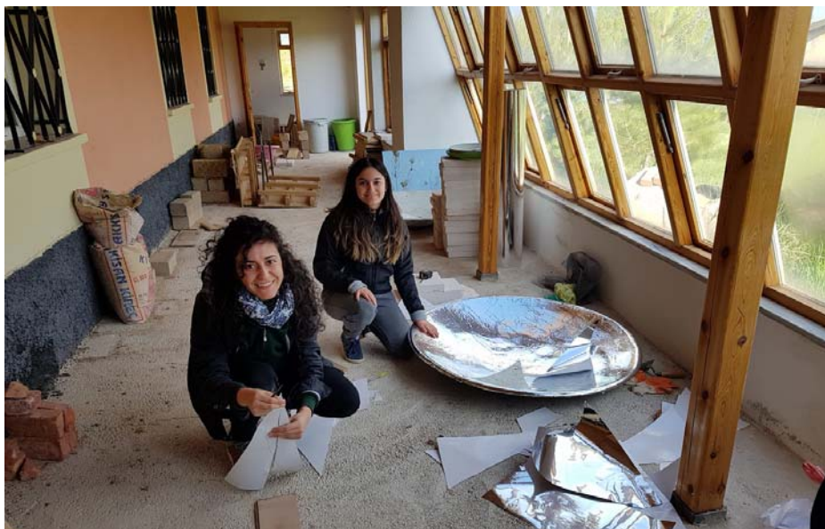
Figure 18. Students covering the solar cooker collector with the new reflective silver foil. (18kekc0229)
