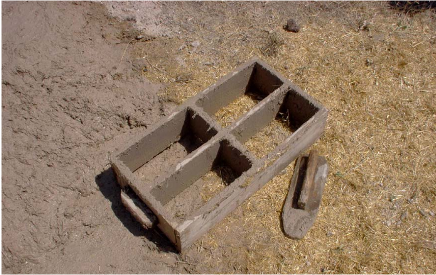
Figure 16: Mud, straw and a simple wooden frame is all that is needed for the production of mud-bricks.
