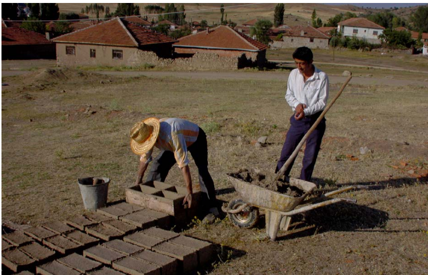
Figure 17: Two villagers producing mud-bricks on a sunny summer day.
