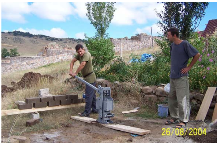
Figure 25. The Parry Brick Press arrived in the village of Şahmuratlı in August 2004 and our visitors, Hasan Çinar and Erkan Alemdar, were very keen to produce the first bricks.
