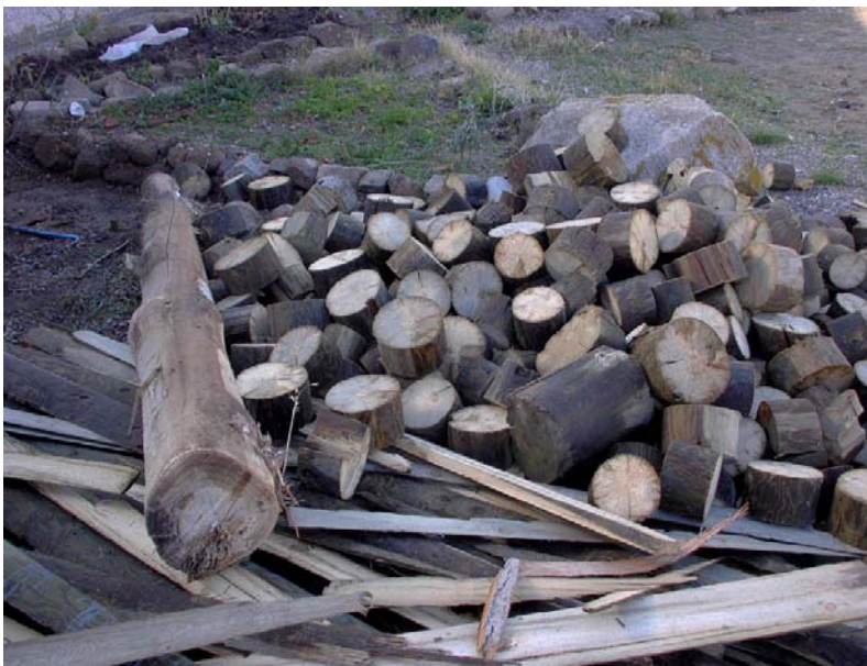
Figure 14. Disused telephone poles from Telekom have been recycled and used in the floor construction. (04kejv0509)
