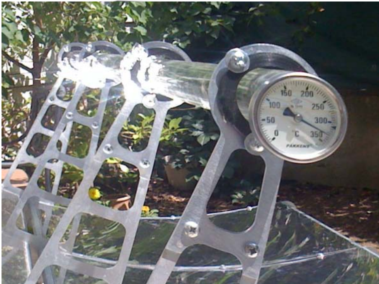
Figure 16. Heat generated inside a glass vacuum tube by the trough parabolic reflector reached almost 350°C
