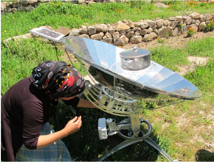
Figure 8. Adjusting the motorized solar cooker. (11kecg0111)
