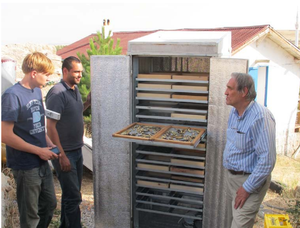
Figure 12. The drying trays are placed on the sliding shelves. The fan is at the bottom of the drying cabinet. (11kecg1106)
