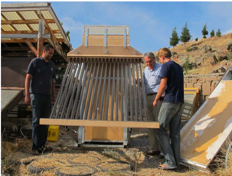
Figure 11. Güner and Korkut Mutaf with the help of Sergey Emeliyanov mounted the motorised solar dryer at the Kerkenes Eco-Center. (11kecg1101)
