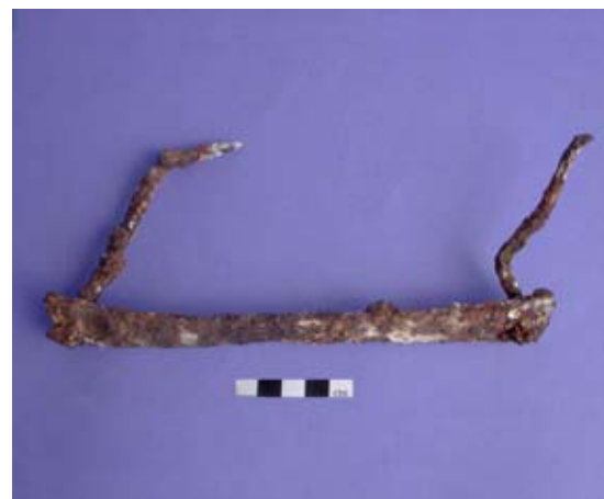
Figure 63. Iron clamp with large nails for fixing into wooden architecture. (03dpjv7106)
