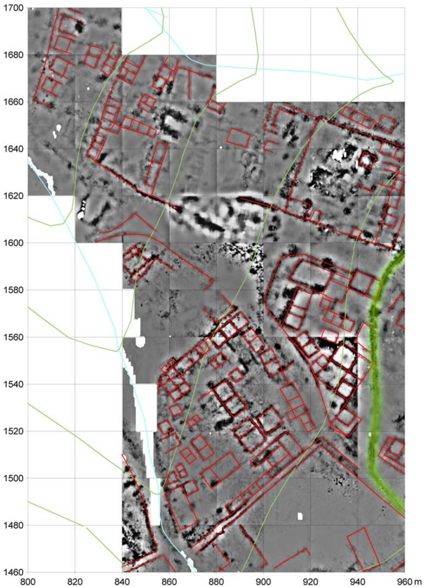
Figure 23. The east-central portion of the resistivity survey with buried walls shown in red and a later enclosure wall in green.
