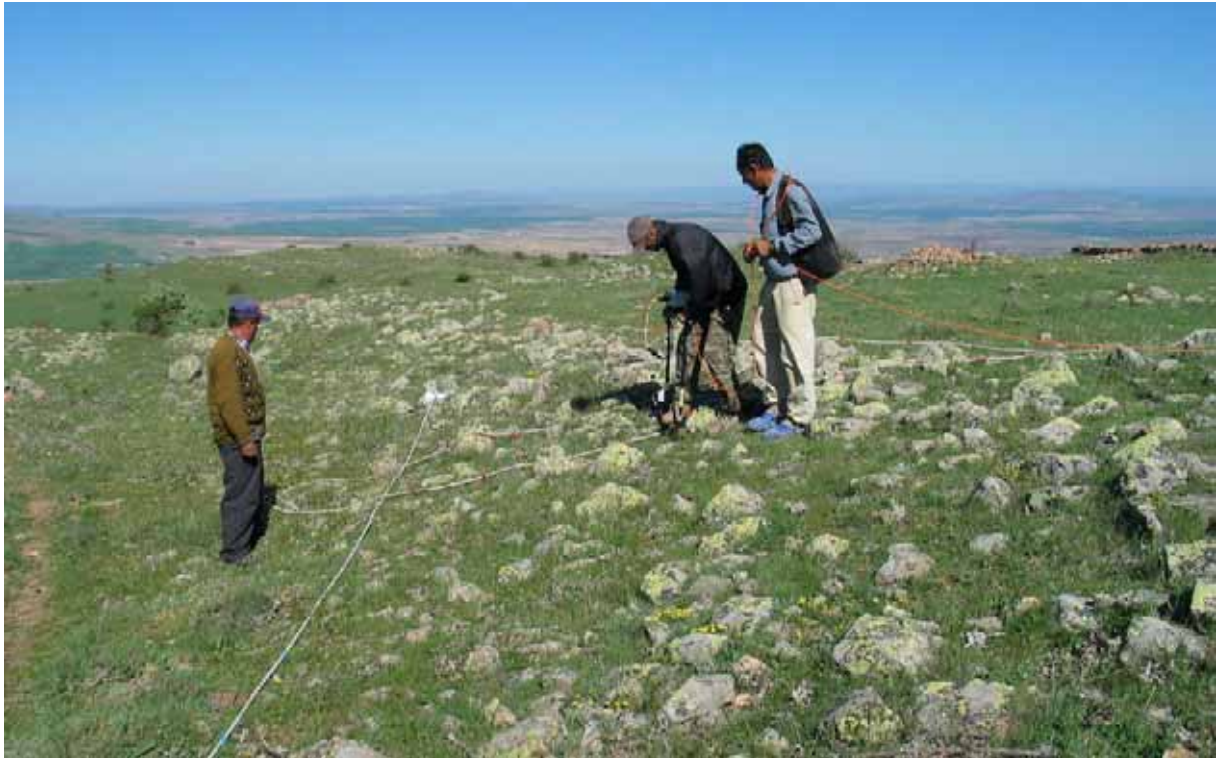
Figure 19. Resistivity survey over stony ground at the Palatial Complex is slow.
