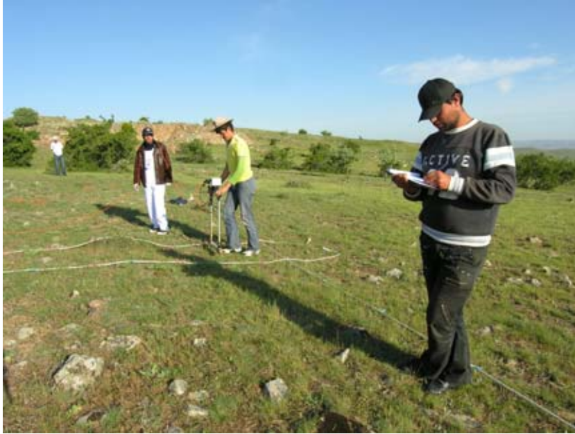
Figure 41. Mehmet Baştürk, Cafer Babayiğit and Muhammed Babayiğit collecting data with a Geoscan RM15 resistivity meter over Area A between the Cappadocia Gate and the Palatial Complex while Fatih Arslan fills grid forms and draws a sketch of each grid. (10dpnc1028)
