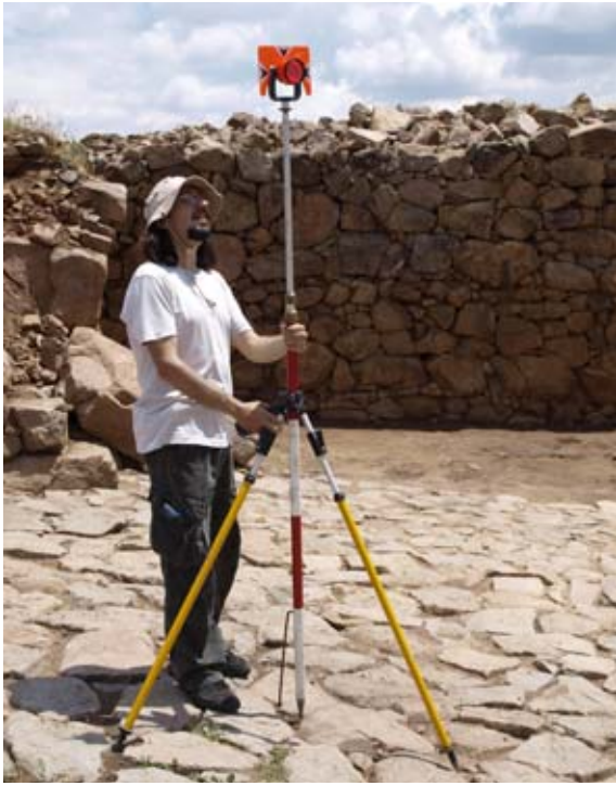
Figure 59. Ahmet Çinici holding the prism over control points surveyed to provide coordinates needed for photorectification. (11dpkc1441)
