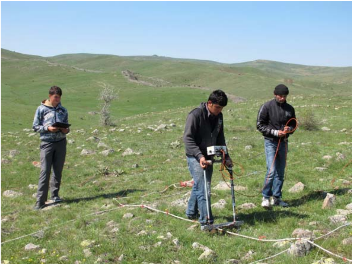
Figure 42. Muhammed Babayiğit, Harun Erciyas and Mehmet Baştürk from Şahmuratlı Village conducting electrical resistance survey with a Geoscan RM15 resistivity meter. (11dpcg0409)
