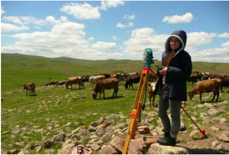
Figure 38. Sema Bağcı repositioning grid corners with a total station for the electrical resistance survey. (11dpkc0146)
