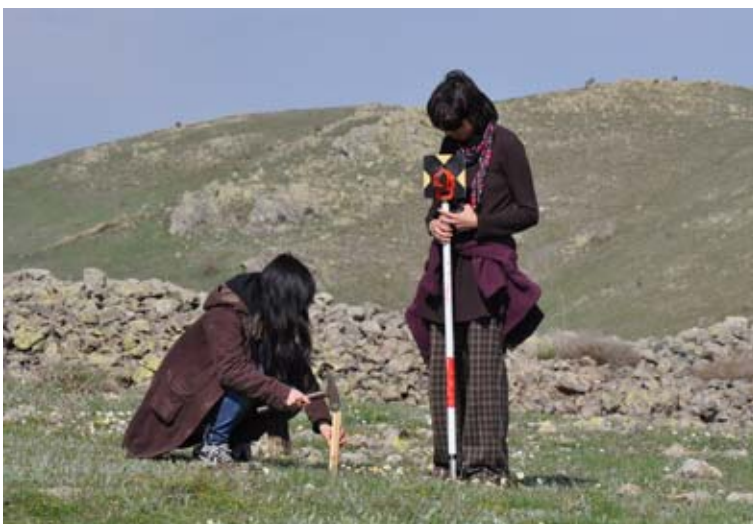
Figure 40. Aslı Oflaz holding the prism while grid corners are marked with wooden pegs and powdered lime. (11dpnd0244)
