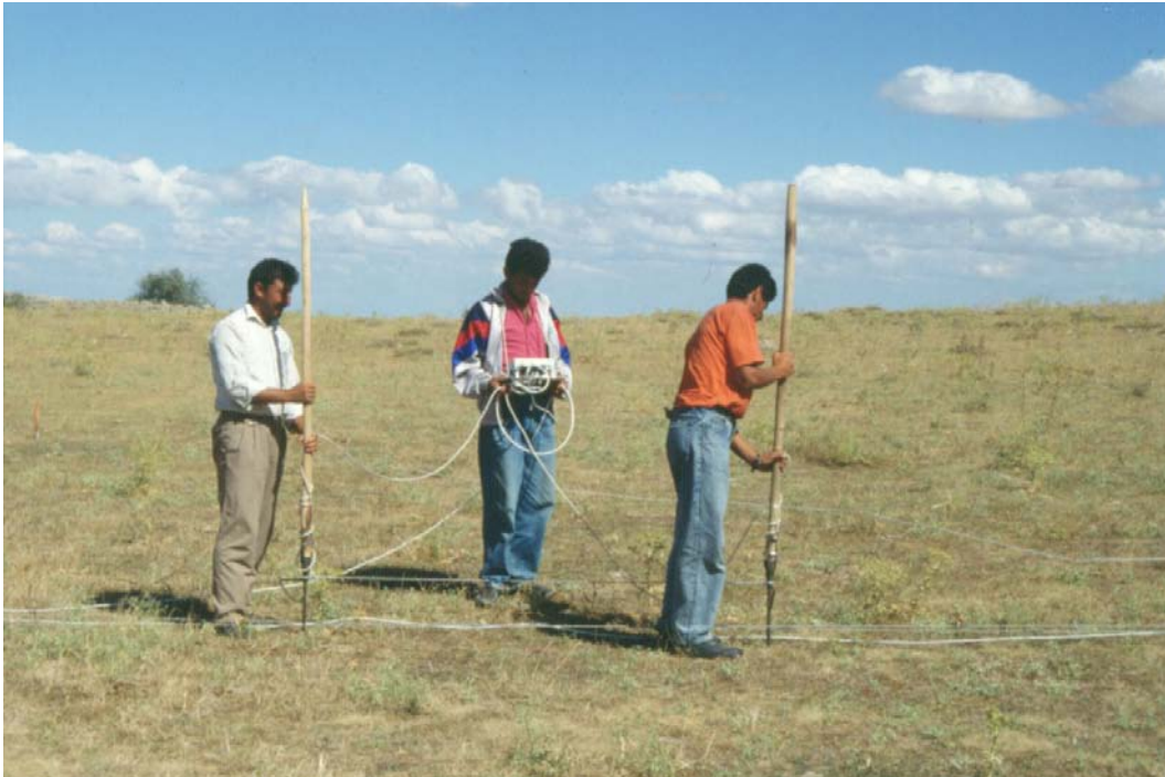
Collecting data with the resistivity meter.
