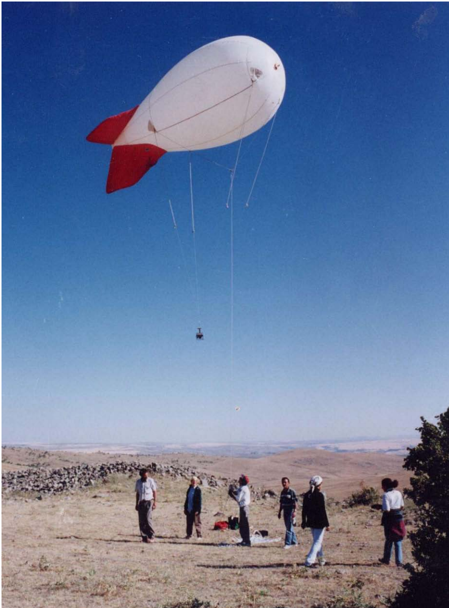
Fig. 2 The blimp going up in ideal, still conditions with the camera in its sling hanging vertically beneath. In these conditions it is possible to fly at high altitudes on a light string. Once a breeze begins a stronger and heavier rope is needed which limits lift. If there is more than a light breeze the blimp is difficult to control, especially when brought close to the ground to change film, and damage may be inflicted on the blimp in a strong wind.
