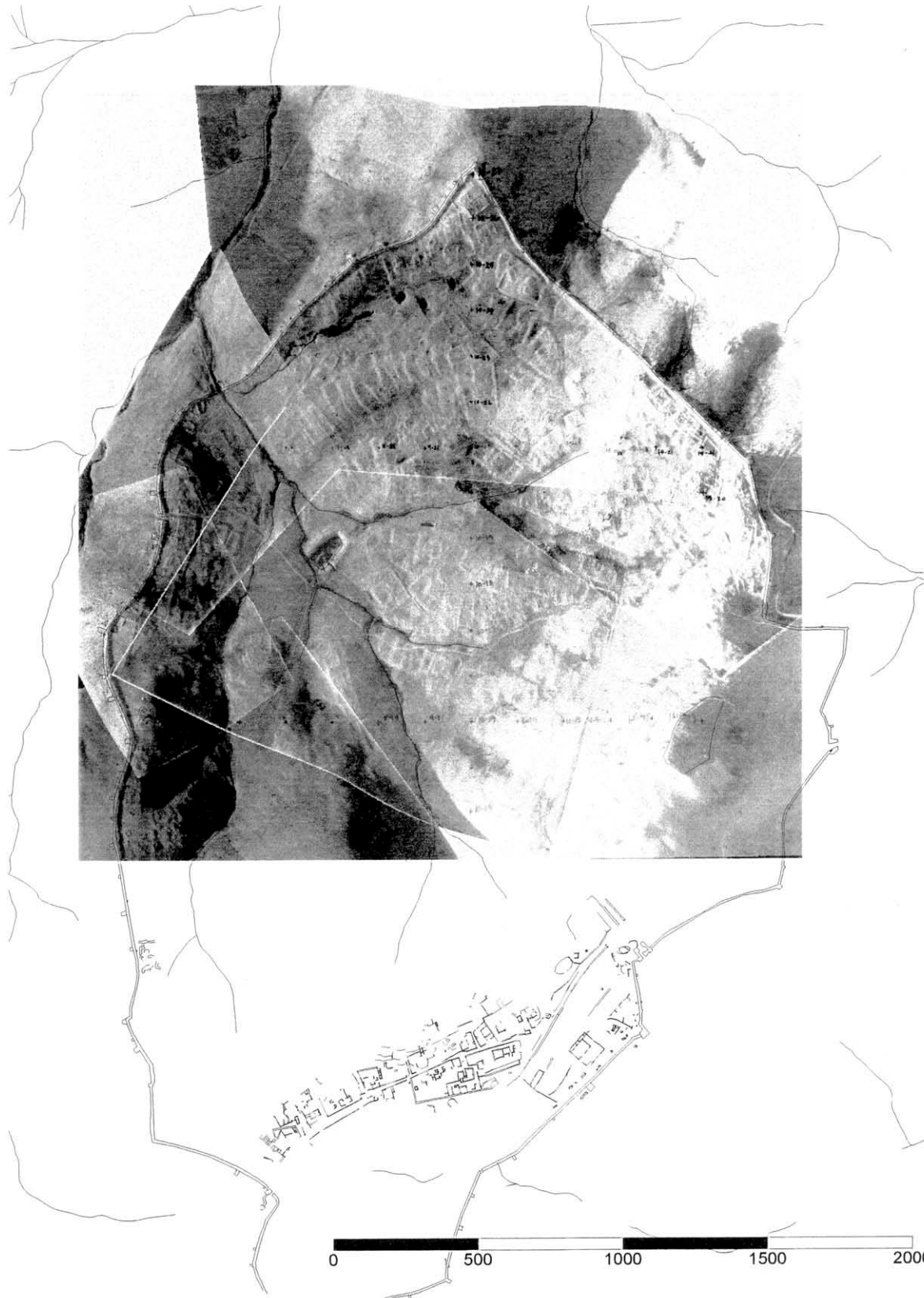
Figure 2. Composite map showing results of photo rectification superimposed on a digitised base map.
