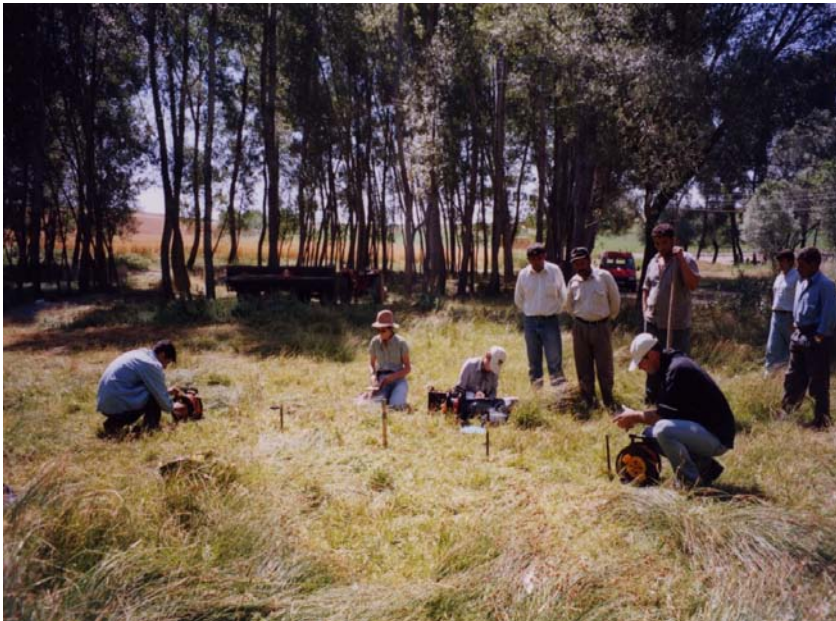
Figure 36: Kuzucuoglu, Ekmekci and Aydin arouse local curiosity while laying out a line across an ancient lake to make a geo-electric profile.
