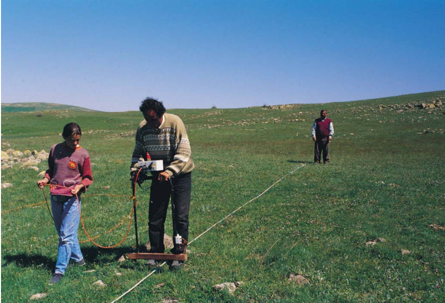
Figure 11: Natalie Summers and Adnan Kilicarslan making the resistivity survey in the spring.
