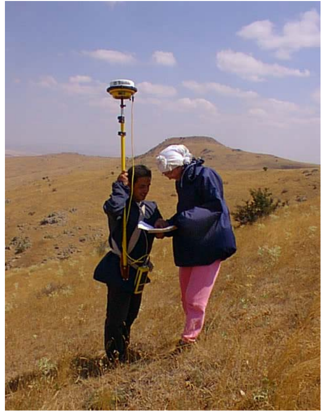
Figure 3: A Trimble 4600LS receiver being used in kinematic GPS survey by Köksal Sanli and Nurdan Atalan.
