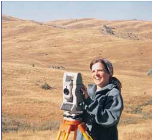
Figure 11: Christine Perrier surveying with a Sokkia Total Station. Şekil 11: Christine Perrier, Sokkia Total Station ile ölçüm yaparken.
