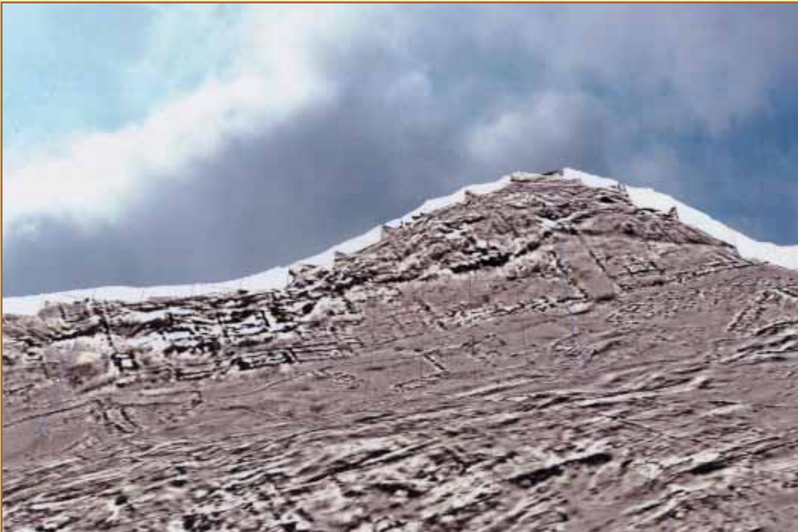
Figure 8: 2-D geophysical image of the northern portion of the site mapped on the GPS terrain model to analyse subsurface remains in 3-D. The city wall is shown as a white strip. Inside the wall, various urban blocks share similar orientation and overlook a small internal valley. The lower area in the centre contains reservoirs and features connected with water resource management.
