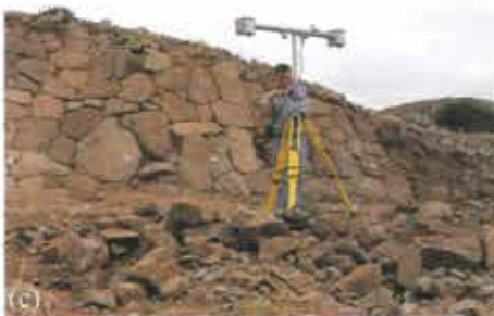
Figure 9: (a) The steeply inclined stone glacis at the Cappadocia Gate is fully preserved in (b) Cleaning the glacis before photography. (c) Kemal Gülcen, of the METU Photogrammetry Group, used stereo photos to m (d) South-East elevation of the Cappadocia Gate drawn from photogrammetry. (e) Placing and removing control points for photogrammetry and rectification re
