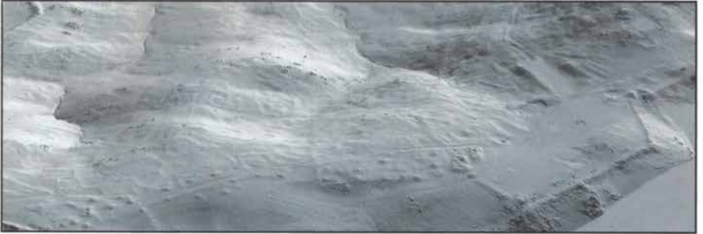
Figure 7: Triangulated Irregular Network (TIN) model of the high southern ridge created in ArcView 3D Analyst from Global Positioning System (GPS) data. Geographic Information System (GIS) uses these models to transform 2D images and maps into 3D data.
