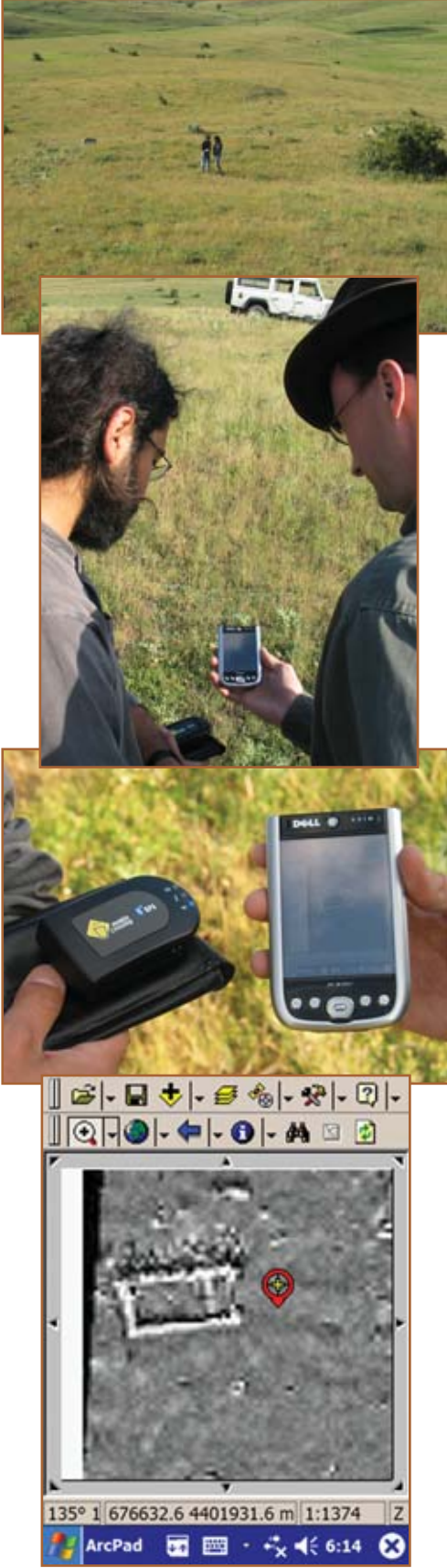
Figure 6. Scott and Tuna verifying geophysical maps with the aid of a handheld GPS receiver and a palmtop.
